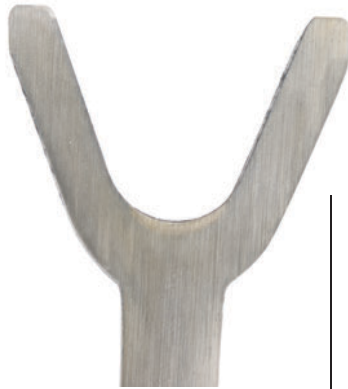
Unretouched photograph of a section cut from a flame hardened McKissick sheave (etched 2-1/2 minutes).
